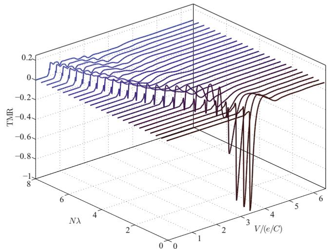
FIG. 3. (Color online) The TMR of an eight-junction array as a function of voltage and the product  $N\lambda$ . The parameters used are  $P = 0.3$ ,  $\tau = 9 \times 10^3 R_0 C$ ,  $[N_0 \Omega]^{-1} = 10^{-3} e^2/C$ , and  $k_B T = 2 \times 10^{-3} e^2/C$ .
