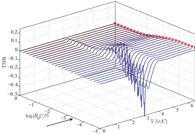
FIG. 4. (Color online) The TMR of an eight-junction array as a function of voltage and spin-relaxation time. The arrow indicates the time between tunneling events close to the threshold voltage ( $e/I$  @  $1.05 \times V_t$ ). The circular symbols shows the large voltage TMR from Eq. (8). The parameters used are  $P = 0.3$ ,  $C_0/C = 2.5 \times 10^{-3}$  ( $\lambda \approx 0.05$ ),  $[N_0\Omega]^{-1} = 10^{-3} e^2/C$ , and  $k_B T = 2 \times 10^{-3} e^2/C$ .
