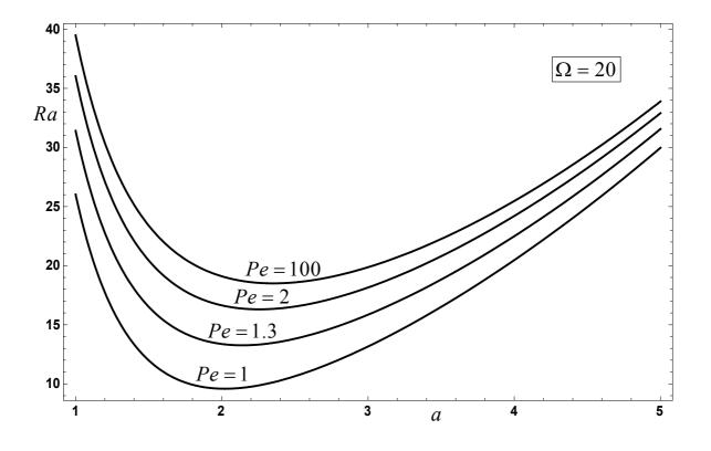
Figure 2: Transverse rolls; neutral stability curves for  $\Omega = 20$ .
