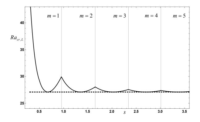
Figure 5: Longitudinal rolls; plot of  $Ra_{cr,L}(s,\Omega)$  versus s for  $\Omega = 10^{-6}$ , where  $s_{cr}(\Omega) = 0.675259$ ; the dashed line corresponds to  $Ra_{cr}(\Omega) = 27.0976$ .
