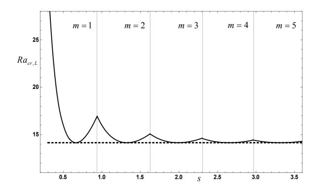
Figure 6: Longitudinal rolls; plot of  $Ra_{cr,L}(s,\Omega)$  versus s for  $\Omega = 30$ , where  $s_{cr}(\Omega) = 0.663036$ ; the dashed line corresponds to  $Ra_{cr}(\Omega) = 14.1493$ .
