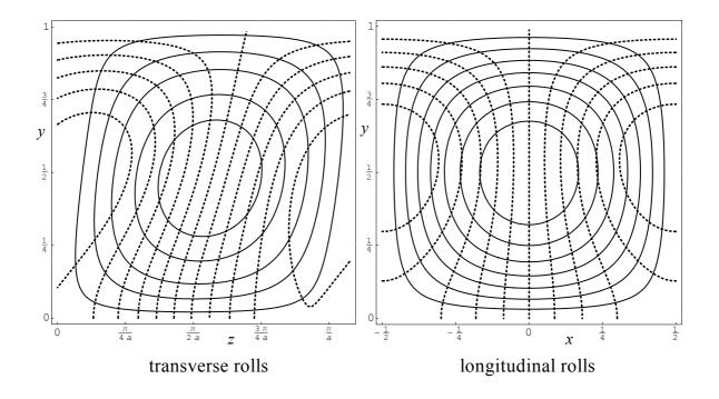
Figure 9: Onset of convection for the case Ra = 0 with Pe = 10 and s = 1/2: streamlines  $\psi = constant$  (solid lines) and isotherms  $\theta = constant$  (dashed lines) with transverse rolls  $(a = 2.40443, \Omega = 60.2103, t = 0)$  and with longitudinal rolls  $(a = \pi, \Omega = 64.8682)$ .
