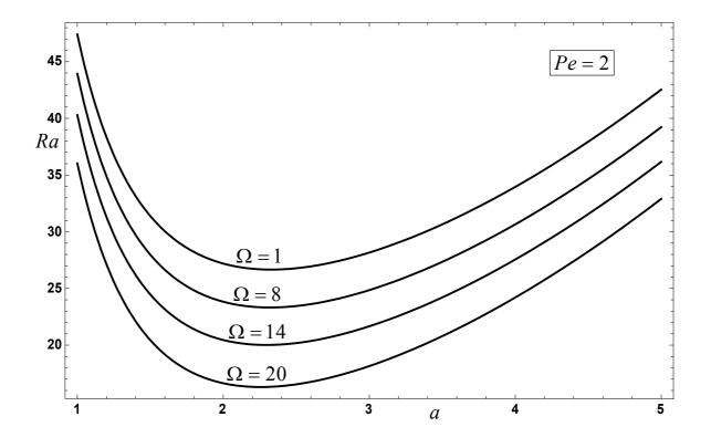
Figure 3: Transverse rolls; neutral stability curves for Pe = 2.
