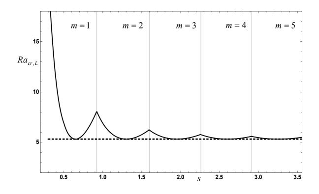
Figure 7: Longitudinal rolls; plot of  $Ra_{cr,L}(s,\Omega)$  versus s for  $\Omega = 50$ , where  $s_{cr}(\Omega) = 0.650634$ ; the dashed line corresponds to  $Ra_{cr}(\Omega) = 5.31993$ .
