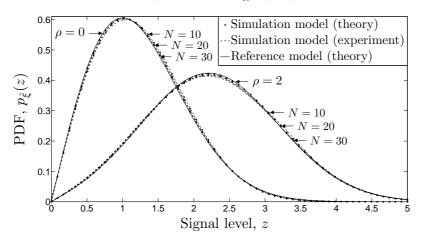
Fig. 3. Comparison of the PDF of Rayleigh ( $\rho = 0$ ) and Rice ( $\rho = 2$ ) processes with the PDF of the envelope of SOC processes  $\hat{\xi}(t)$  designed by using the EMEDS with  $N \in \{10, 20, 30\}$  ( $\sigma_0^2 = 1, f_{max} = 91$  Hz).
