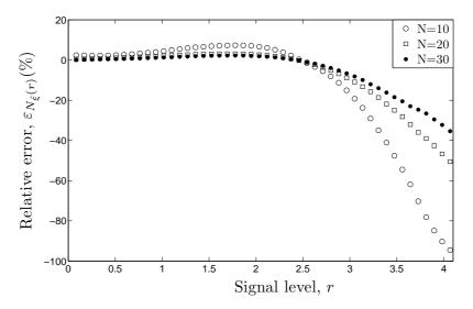
Fig. 6. Relative error  $\epsilon_{N_{\xi}}(r)$  of the LCR of SOC processes designed by using the EMEDS with  $N \in \{10, 20, 30\}$  ( $\sigma_0^2 = 1, f_{\text{max}} = 91$  Hz,  $\rho = 0$ ).
