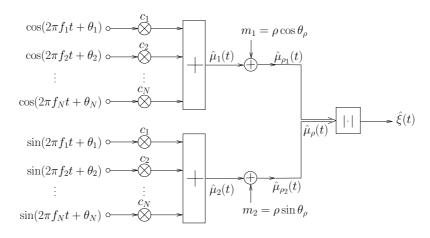
Fig. 1. Structure of an SOC simulation model for Rice fading channels.
