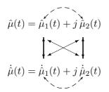
Fig. 2. Illustration of the correlation between the inphase and the quadrature component of SOC processes and their respective time derivatives (intracorrelation:  $\leftarrow - \rightarrow$ ; intercorrelation:  $\longleftrightarrow$ ).
