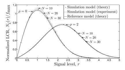
Fig. 4. Comparison of the normalized LCR of Rayleigh ( $\rho = 0$ ) and Rice ( $\rho = 2$ ) processes with the normalized LCR of SOC processes designed by using the EMEDS with  $N \in \{10, 20, 30\}$  ( $\sigma_0^2 = 1, f_{max} = 91$  Hz).
