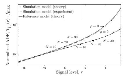
Fig. 5. Comparison of the normalized ADF of Rayleigh ( $\rho = 0$ ) and Rice ( $\rho = 2$ ) processes with the normalized ADF of SOC processes designed by using the EMEDS with  $N \in \{10, 20, 30\}$  ( $\sigma_0^2 = 1, f_{max} = 91$  Hz).
