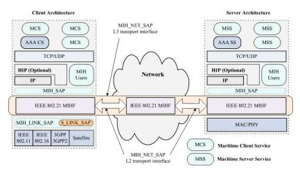
Fig. 2. Maritime Communication Architecture Protocols Stack
