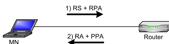
Figure 7.6 – A MN can request the router for a new address using RPA destination option.
