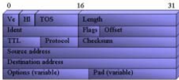
Figure 2.1: The IPv4 header.
