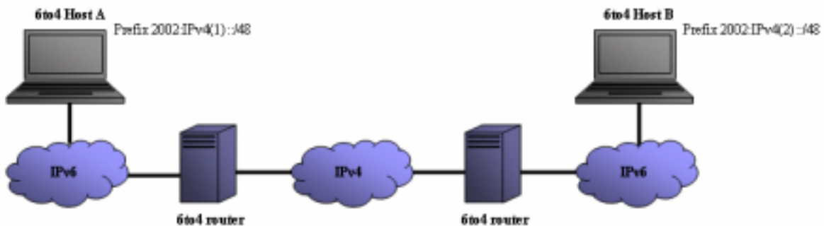
Figure 4.5: Communication between two 6to4 hosts.
