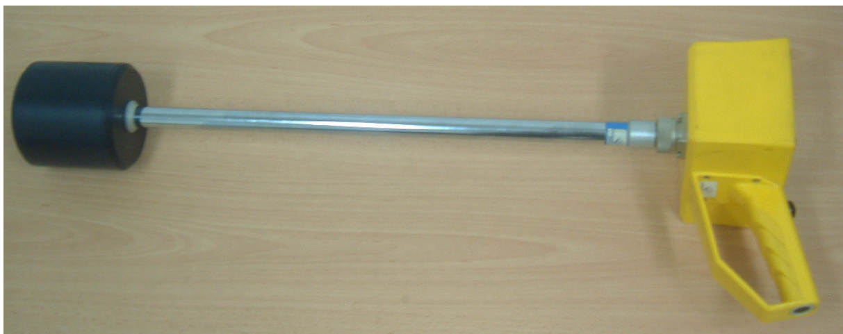
Figure 3.2 – The reader and antenna of the old RFID system
