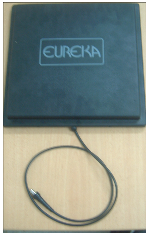
Figure 10.3 – Avonwood's Eureka RFID antenna
