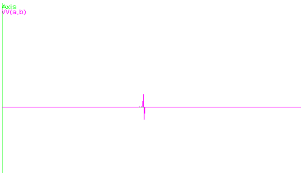
Graph 27: The transformed signal of simple line using Haar
