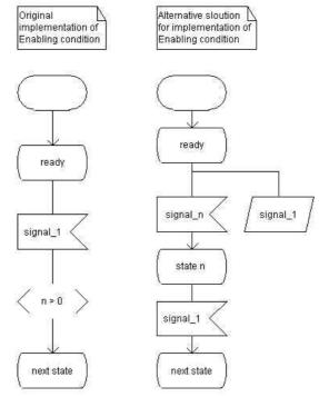
Figure 13 Enabling condition SDL
