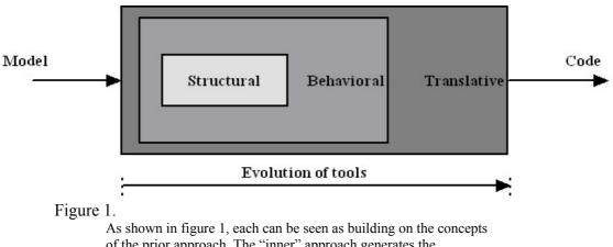
As shown in figure 1, each can be seen as building on the concepts of the prior approach. The "inner" approach generates the framework code for the object structure of a system. Newer approaches model behaviour sufficiently to enable generation of system functionality. The most recent approach adds an architecture model that enables user control of all generated code.
