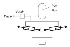
Fig. 6 Pendulum bar stabilizing system circuit
