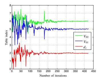
Fig. 14 Development of the three discrete design variables with constant  $\epsilon$
