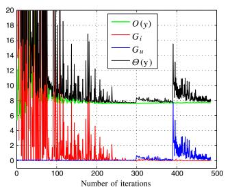
Fig. 11 Development of the objective function  $O(\mathbf{y})$ , side constraints violation  $G_i$ , integer evaluation  $G_u$  and the augmented objective function  $\Theta(\mathbf{y})$
