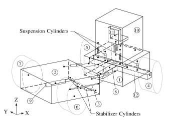
Fig. 2 Hydrema 912DS articulated dump truck consisting of 12 bodies
