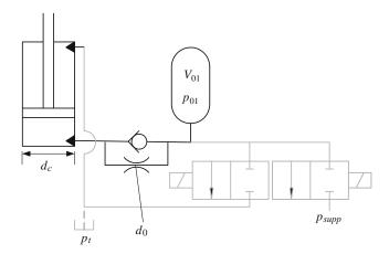
Fig. 5 Characteristics of direction valve and orifice
