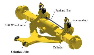
Fig. 4 Front axle suspension design
