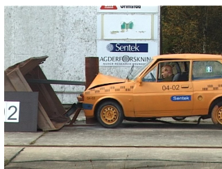
Fig. 6. Car during a collision (Robbersmyr (2004))
