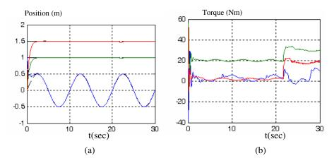
**Fig. 4.** Performance of adaptive control based on wavelet networks for system with inconstant parameters: (a) Tracking curve, (b) Controller output- $\tau(t)$
