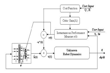
Fig. 1. Adaptive control design based on wavelet networks
