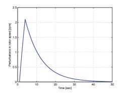
Fig. 15. Response in rotor speed without any control
