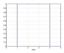
Fig. 13. Step signal for disturbance modeling
