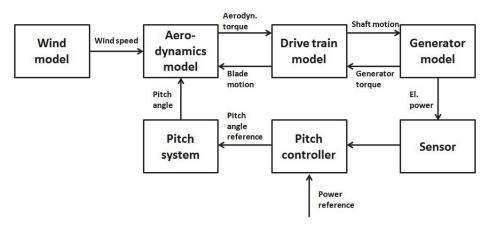
Fig. 1. WT subsystems with corresponding models
