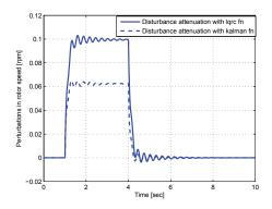
Fig. 17. Comparison of rotor speed for similar control effort while applying kalman and lgrc functions in MATLAB
