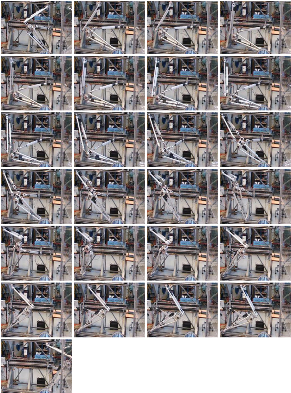
Fig. 5 The reconfiguration sequence of 25 positions on the 5-DOF Gantry-Tau at the University of Agder as optimised by CPLEX (sequence moves from left to right and top to bottom )
