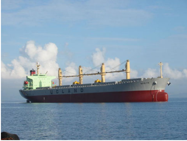
Fig. 3. M/V Rosita managed by Uglund Marine Services AS is a typical bulk carrier. The engine of 7.8 MW represents a large source of waste heat. Source: Uglund.
