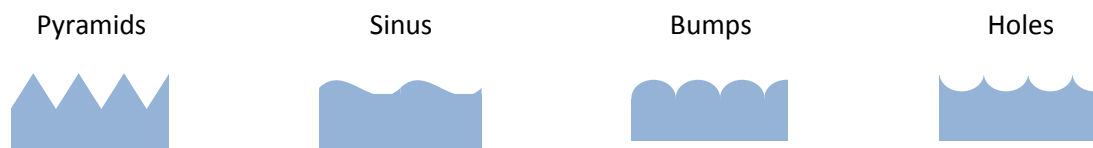
Figure 71: A selection of common texture patterns used on glass surfaces to reduce reflectivity. Pyramids, sinus-shape, bumps and holes are simple geometrical features that can be replicated in ray tracing simulations.
