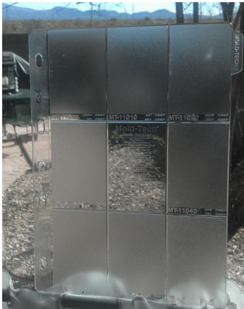
Figure 81: Image of rough glass produced by Mold-Tech with different RMS roughness values. The glass appears as matt/ground glass as the surface scatters the light. Source: Correspondence with M. Gauvin from TracePro.
