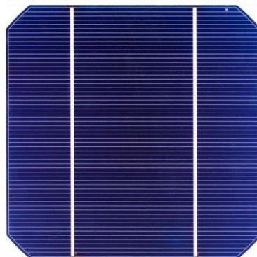
Figure 32: Front surface of a mono-crystalline solar cell with two bus bars and fingers [48].
