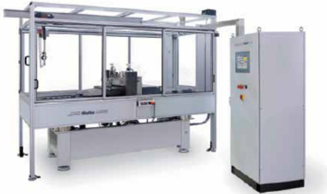
Figure 9: DSM's pilot slot-die coating line
