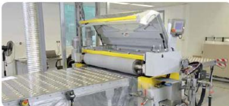
Figure 8: Roll coating unit in DSM's Technology Development Center
