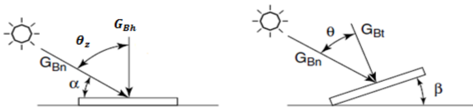
Figure 4.5: Beam radiation on horizontal and tilted surface [33].
