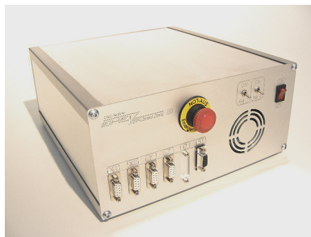
Figure 3.4: Control Box for the mill
