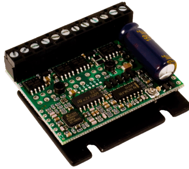
Figure 2.8: G251 Stepper Motor Driver with 1/10 microstepping and 3.5 amp capability
