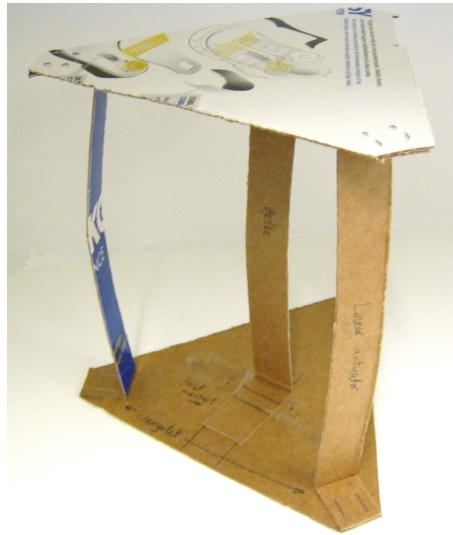
Figure 3.2: Cardboard mockup of linear actuator tilting table
