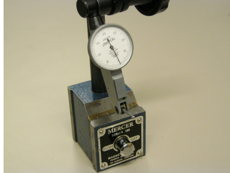
Figure 3.28: Dial Gauge used to measure the backlash
