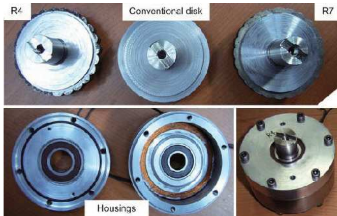
Figure 3.2. 1 MR brake structure with the form of rotary disks
