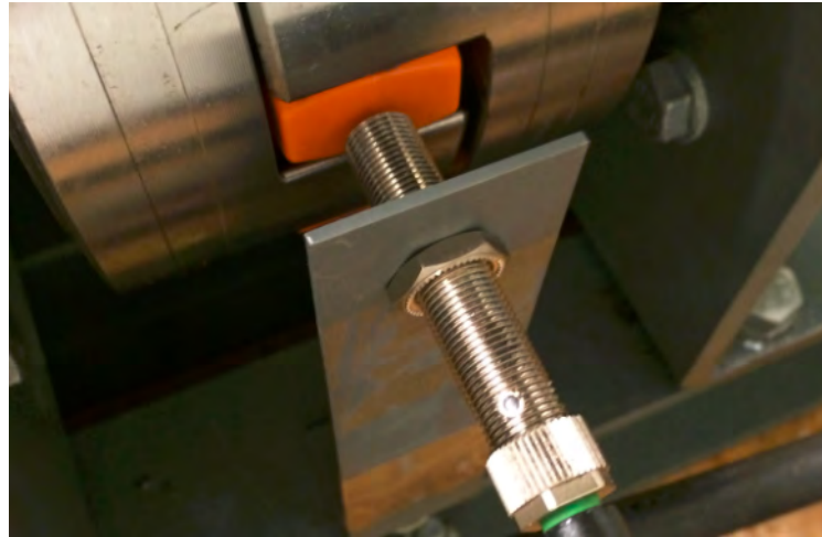
Figure 5.4: Inductive sensor fitting. Here shown when the output signal is false.
