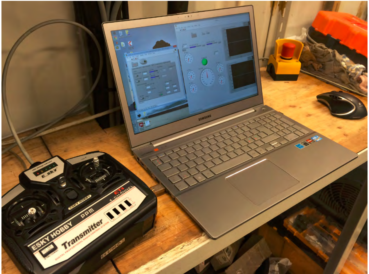
Figure 5.2: Laptop running LabVIEW for monitoring and control of the load circuit. The hand held controller to the left is used to set speed and load references.
