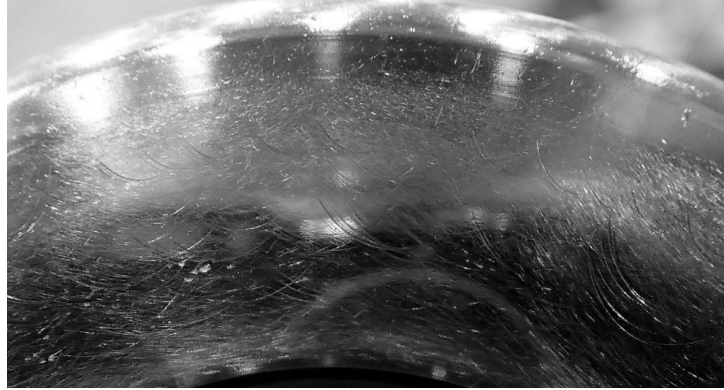
Figure C.2: Scoring on roller end of tapered roller bearing
