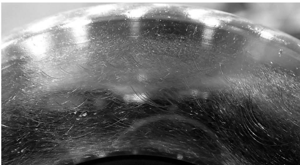
Figure E.1: Wear on roller end of offshore drilling machine bearing.
