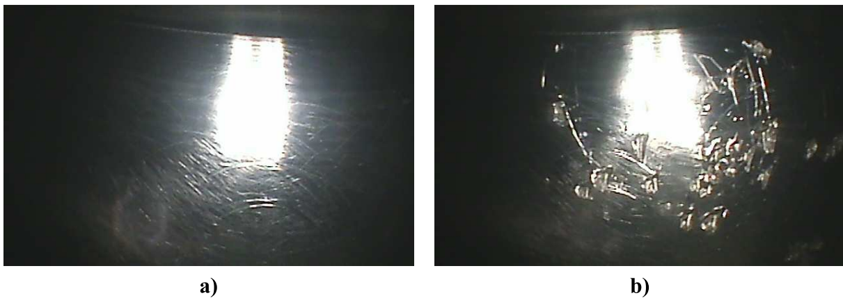
Figure 2.3: Artificially damaged top drive bearing. a) Boroscope image of roller end scratches on top drive main bearing. b) Boroscope image of artificially damaged bearing.
