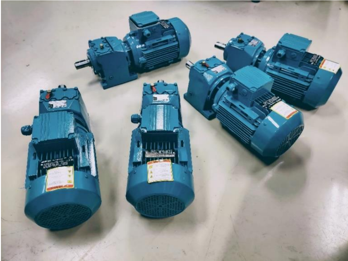
Figure 1.1: Gearbox based motors in an electric powertrain
