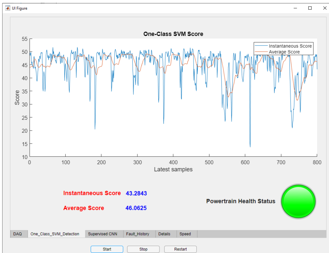
Figure F.17: One-class SVM fault detection interface.
