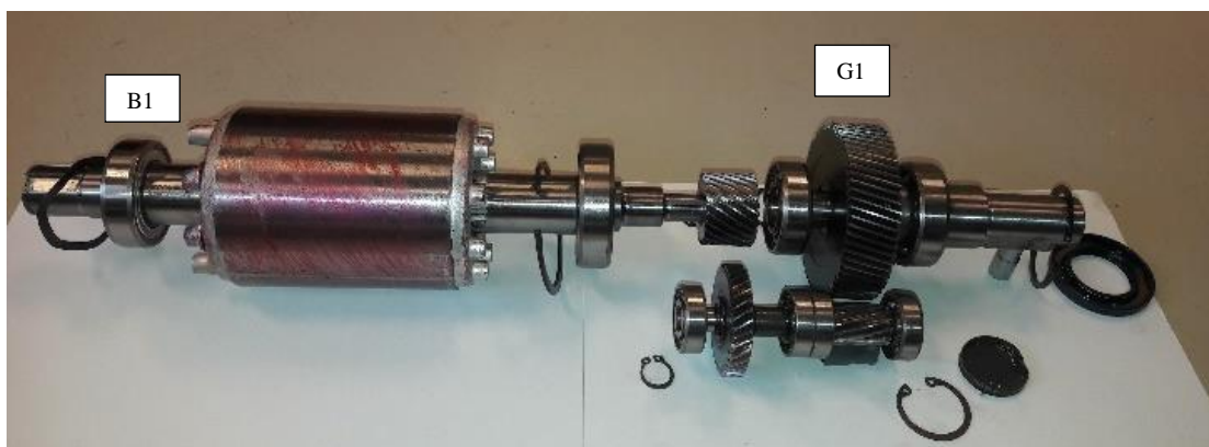
Figure D.7: The internal components of the electric powertrain.
