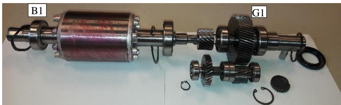
Figure E.5: The internal components of the electric powertrain.
