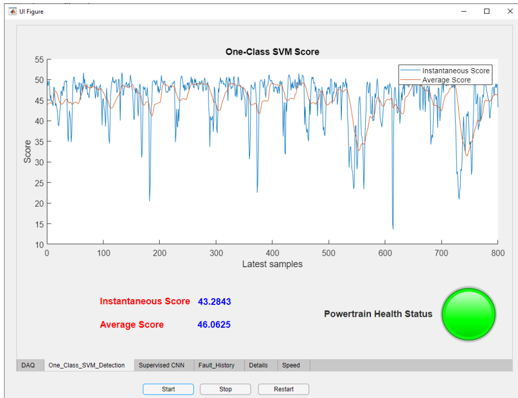
Figure 6.4: One-class SVM fault detection interface.
