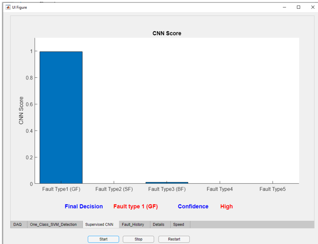
Figure F.18: CNN fault score and decision-making interface.
