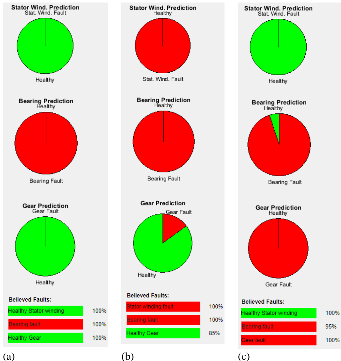
Figure E.8: A snap shot of online fault diagnosis system performance (a) bearing fault (b) stator winding and bearing faults (c) bearing and gear faults.
