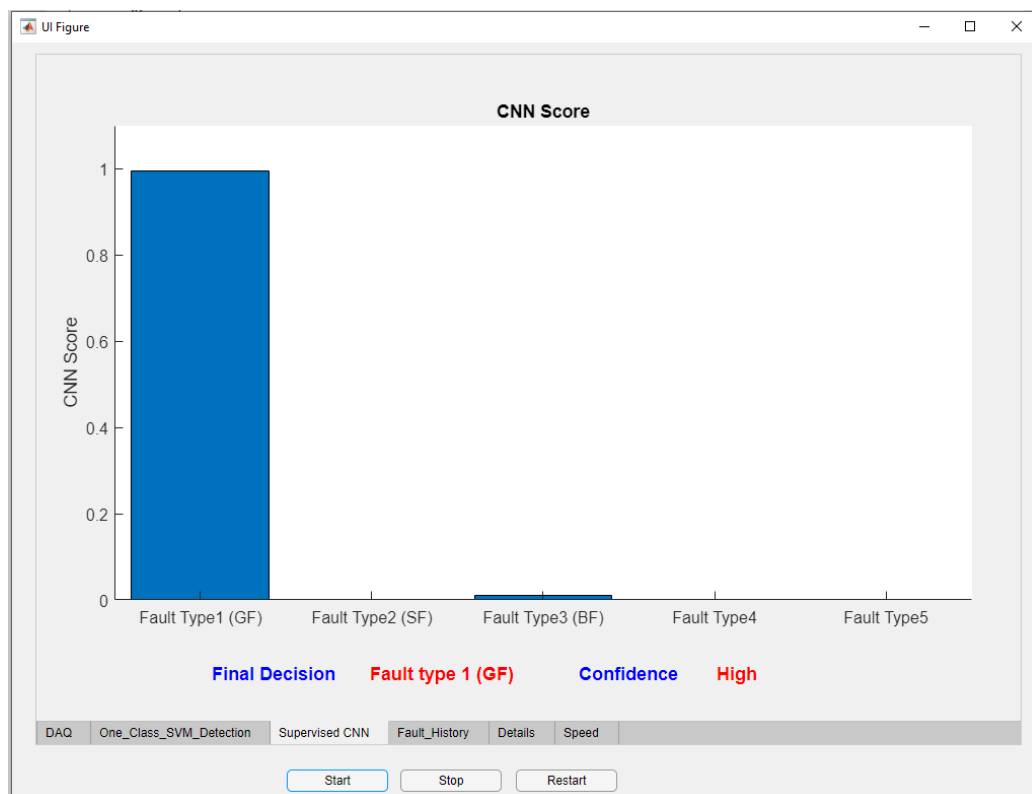
Figure 6.5: CNN fault score and decision-making interface.
