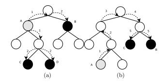
Fig. 3: Fig. 3a shows the neighborhood for the TTO-SOM. Here nodes B, C and D are equidistant to A even though they are at different levels in the tree. Observe that non-leaf nodes may be involved in the calculation. Fig. 3b shows the case for the ET, where nodes B and C are equidistant to A. In the ET, the definition of the distance pertains only to leaf nodes.
