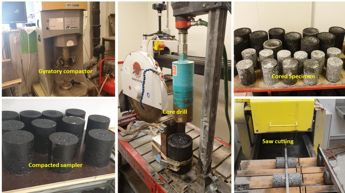
Figure 3.2: Specimen fabrication
