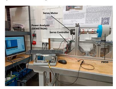
cating various wind conditions and evaluating the generator's behavior under different operational scenarios. Figure 3 shows the WTG test bench.
