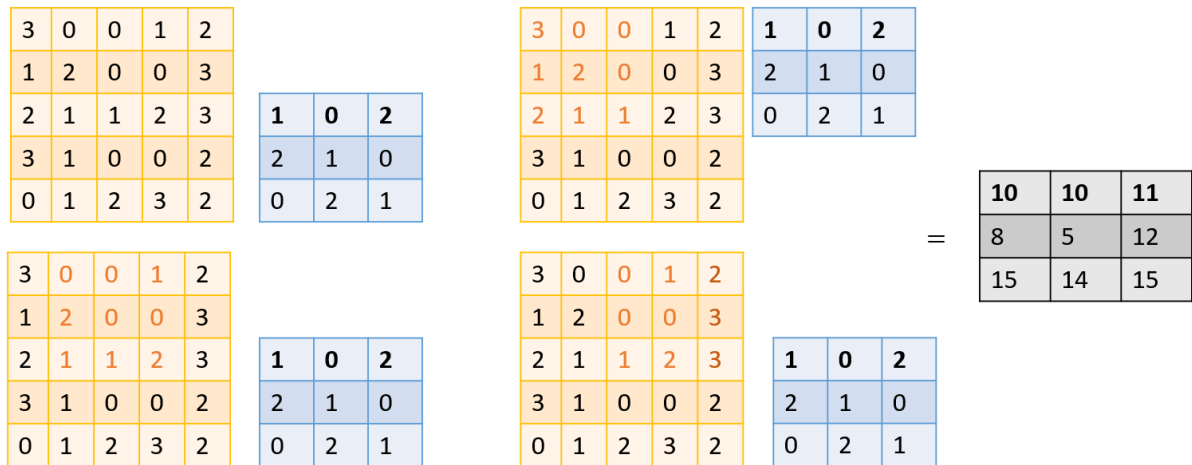
Figure 2.18: Convolution with 3x3 matrix Kernel
