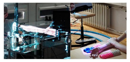
Figure 4. Scanning of the patient, (a) left arm—mechanized rig, (b) right arm—manual scan.
