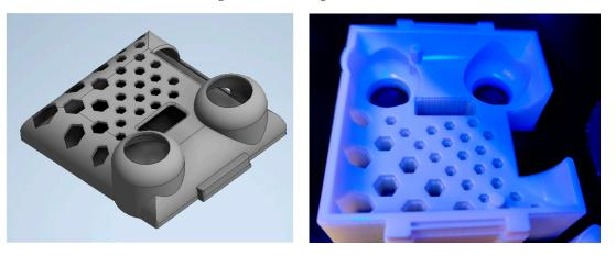
DraftWhite material (UV resin), with layer thickness of  $18 \mu m$ . Design of this housing and its manufacturing is shown in Figure 8.
