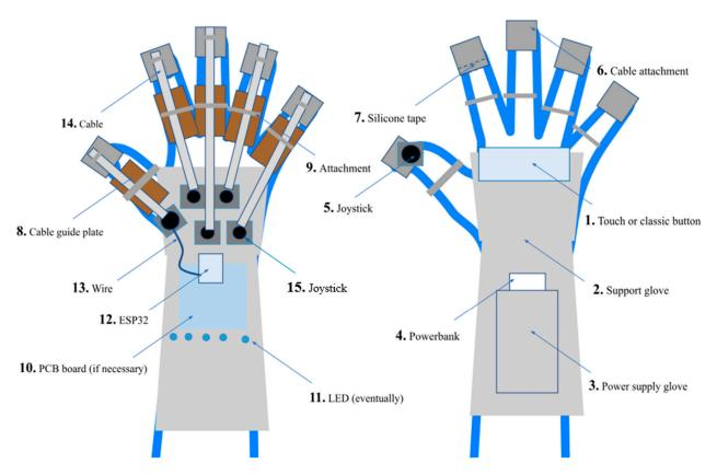
Figure 7. Controller schematic, indicating the most important components.
