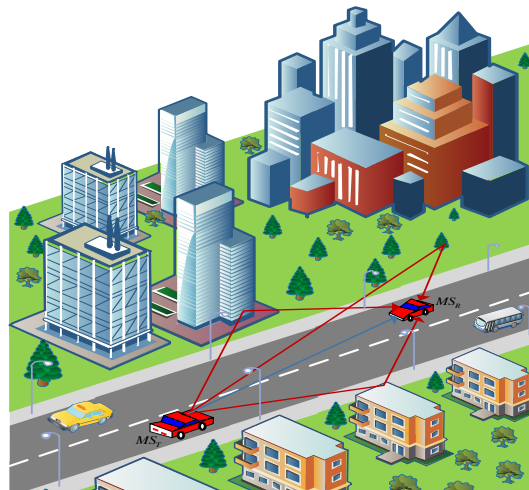
Figure B.1: A typical propagation scenario along a straight street in urban areas.
