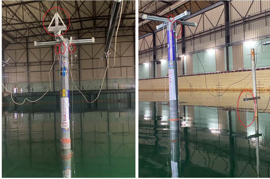
(a) Spar 1 with all the instrumentation.
