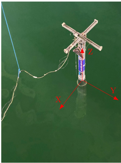
Figure 2: Top view of the model with the aluminum structure, including the instrumentation cables.
