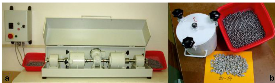
Fig. 2 Diagram of micro-Deval setup (a) and standard 10/14-mm aggregates specimen, steel drum, and 5-kg spherical steel balls (b) (adapted from Durmeková et al. (2019))
