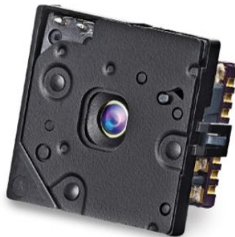
Figure 3.2: FLIR Lepton 3.5. The figure is taken from their webpage. 2
