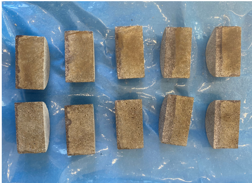
Figure 6.5: Test specimens with visible silver chloride precipitation
