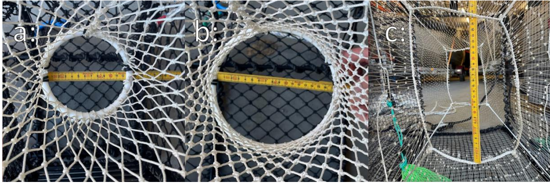
Figure 3: Entrance size of the three trap types a) Small trap entrance (120mm), b) Medium trap entrance (180mm) and c) large trap entrance (270mm, fully expanded)
