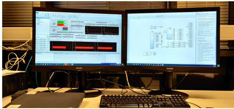
Figure 3.7: Real-time interface of dSpace Control Desk and Matlab/Simulink.
