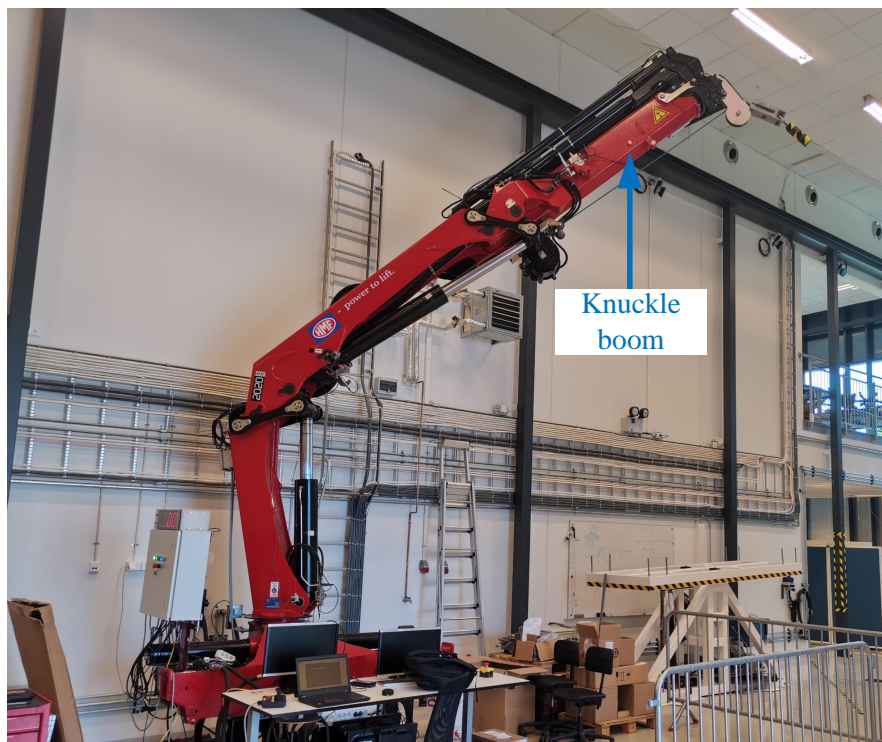
Figure 22. HMF 2020K4 loader crane in the laboratory.
