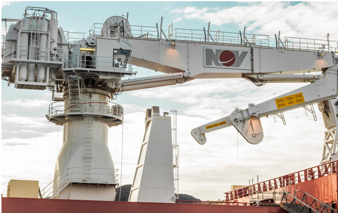
Figure 1. Typical offshore knuckle boom crane, courtesy of National Oilwell Varco©.
