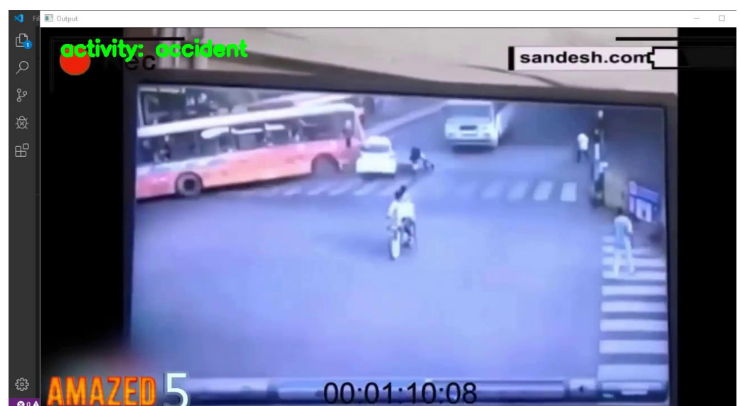
Figure 14. Result captured by test 1. In this scenario, the resolution of the camera was too low, but the viewing angle was in the right direction.
