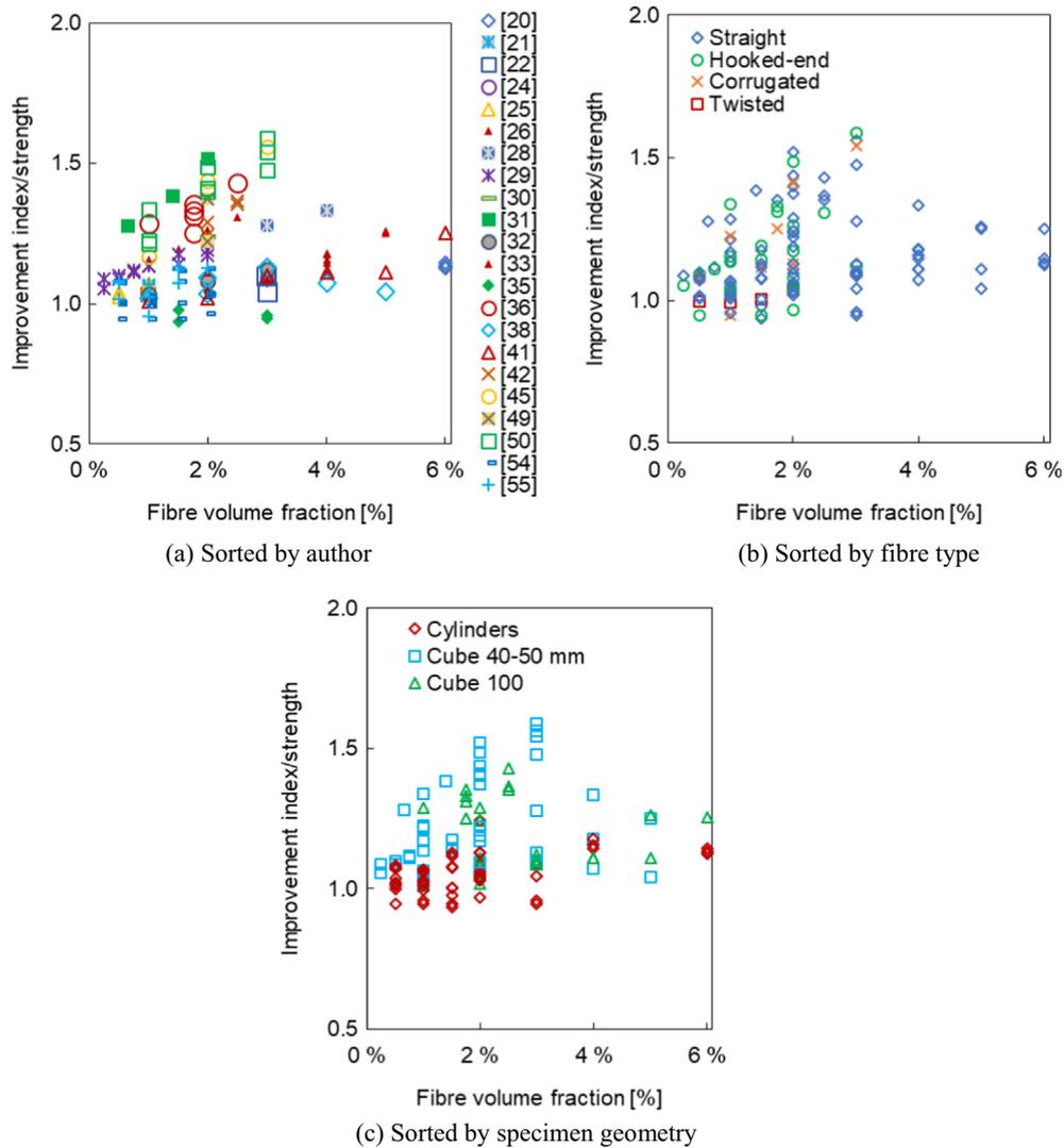
**Fig. 3.** Improvement index for compressive strength of fibre reinforced UHPC as a function of fibre content. The improvement index is calculated following Pakravana & Ozbakkaloglu [73]: the value of fibre reinforced concrete relative to that of the unreinforced concrete sample. The data is obtained from all relevant research papers in Table 2.
