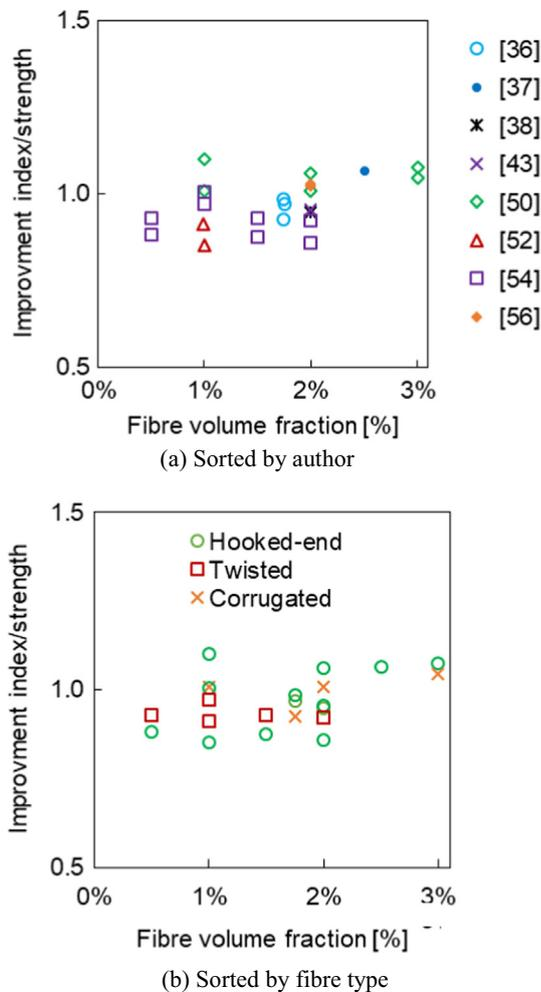
**Fig. 4.** Improvement index for deformed fibres on compressive strength as a function of fibre content. The improvement index is calculated for different deformed fibres relative to 13 mm straight fibres for corresponding volume fractions. The data is obtained from all relevant research papers presented in Table 2.
