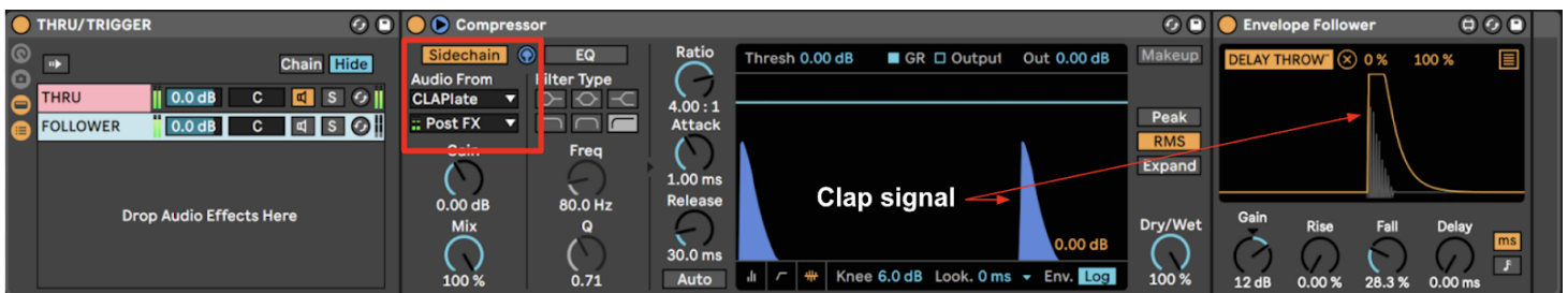
Figure 23: An illustration of the sidechain listen function accepting a signal from an external source (the clap track), which is being interpreted by the envelope follower. The red arrows have been added to indicate both the source track and the resulting envelope curve.
