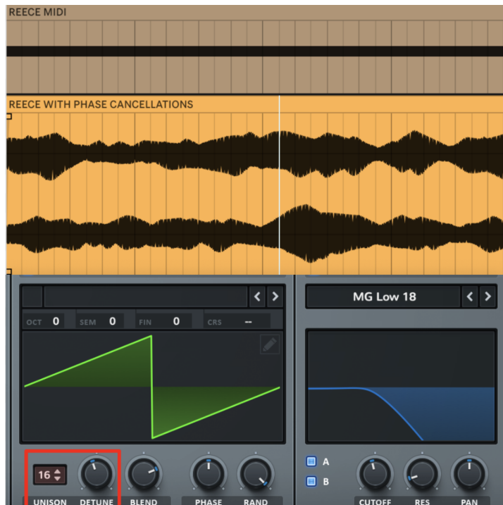
Figure 13: Filtered Saw wave with 16 detuned oscillators illustrating more complex cancellations. A low pass filter has also been added in this example to drastically reduce high frequency content, a staple in this kind of bass sound.
