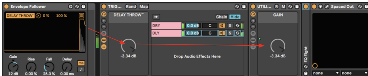
Figure 25: A more comprehensive overview over what the envelope follower is controlling.
