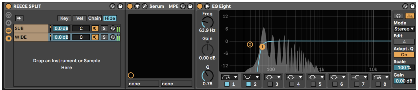
Figure 17: The “WIDE” section playing the original detuned saw with an equalizer removing the fundamental frequency.
