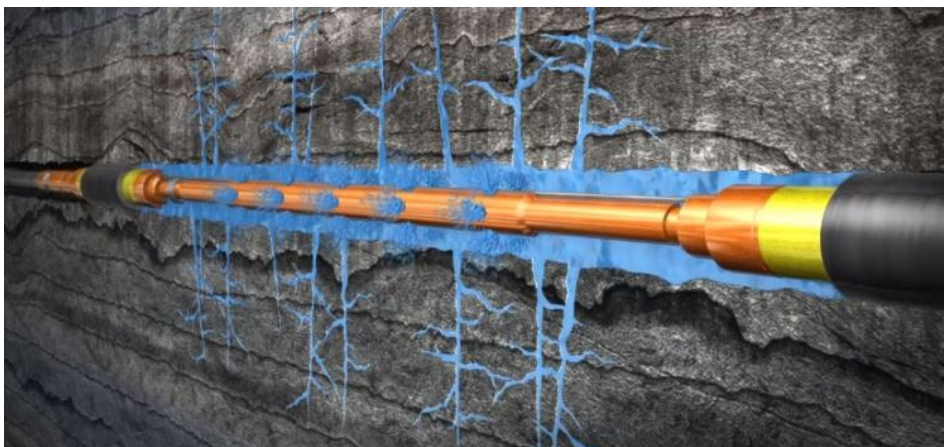
Figure 4-21: Illustration of CT with straddle packer assembly (TAM International, 2013)
