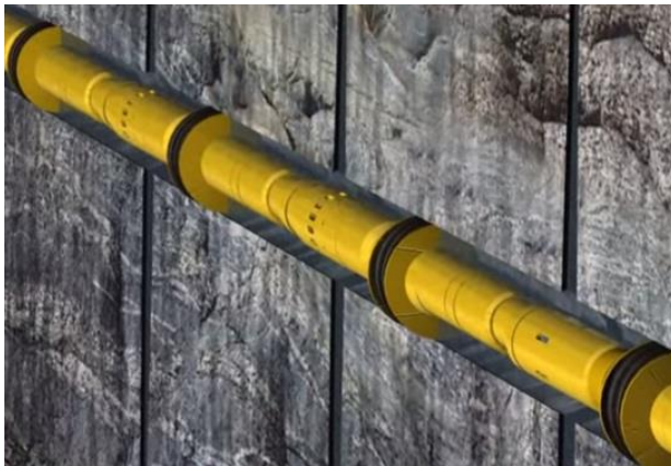
Figure 4-8: Illustration of an open-hole completion, with a sleeve and packers (Baker Hughes)
