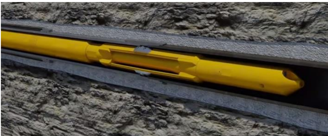
Figure 4-17: Coiled tubing used to slide a sleeve - Mechanical activation (Baker Hughes, 2010)
