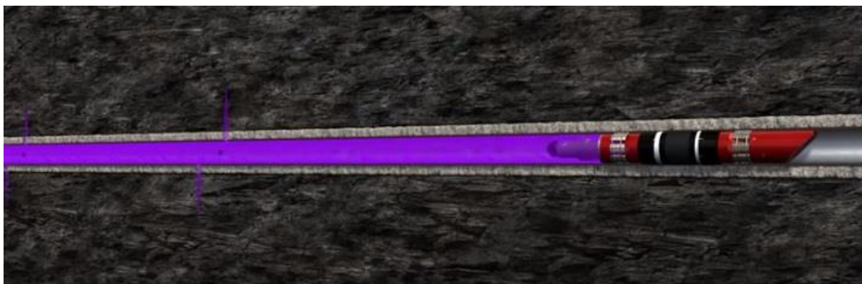
Figure 4-13: Illustration showing a released ridge plug making zonal isolation, plug and perf technique (Weatherford, 2014)
