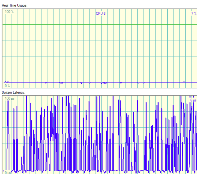
Figure 4.28: Latency and core usage of TwinCAT using a shared core at 80% usage limit
