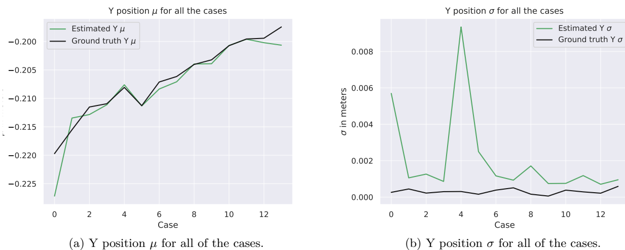
Figure 6.13: Y position cases for the 2 meter standstill test.
