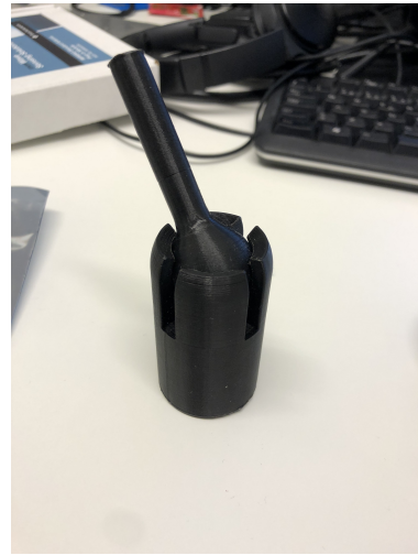
Figure 5.2: Ball-and-socket joint as a part of the bracket
