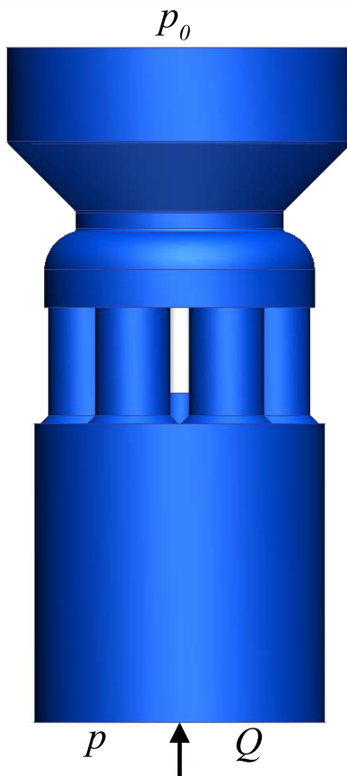
Figure 3.20: CFD model of fluid volume from the fire monitor with boundary conditions.
