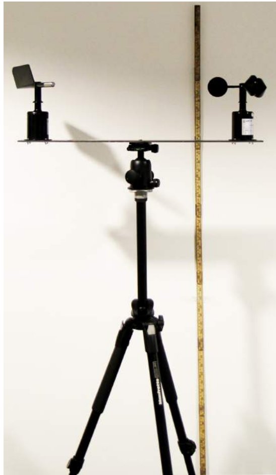
Figure 3.15: Sensor rack with 2 m yardstick.
