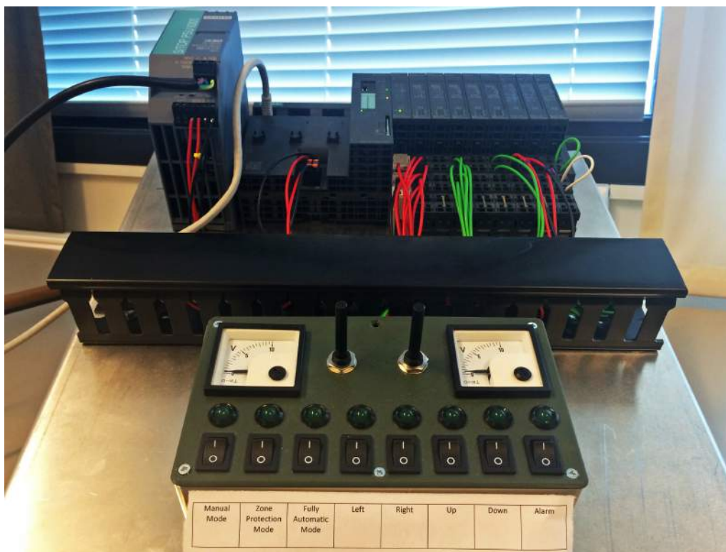
Figure 3.39: PLC with analog and digital inputs.
