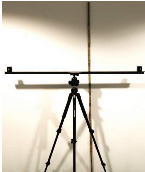
Figure 3.31: Camera rack with 2 m yardstick.
