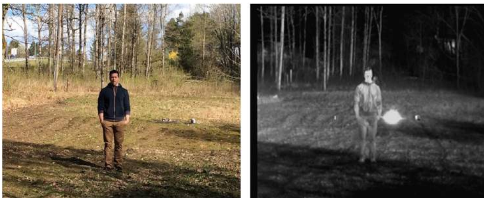
Figure 2.14: Color image versus IR. The heat source is a small wooden fire.
