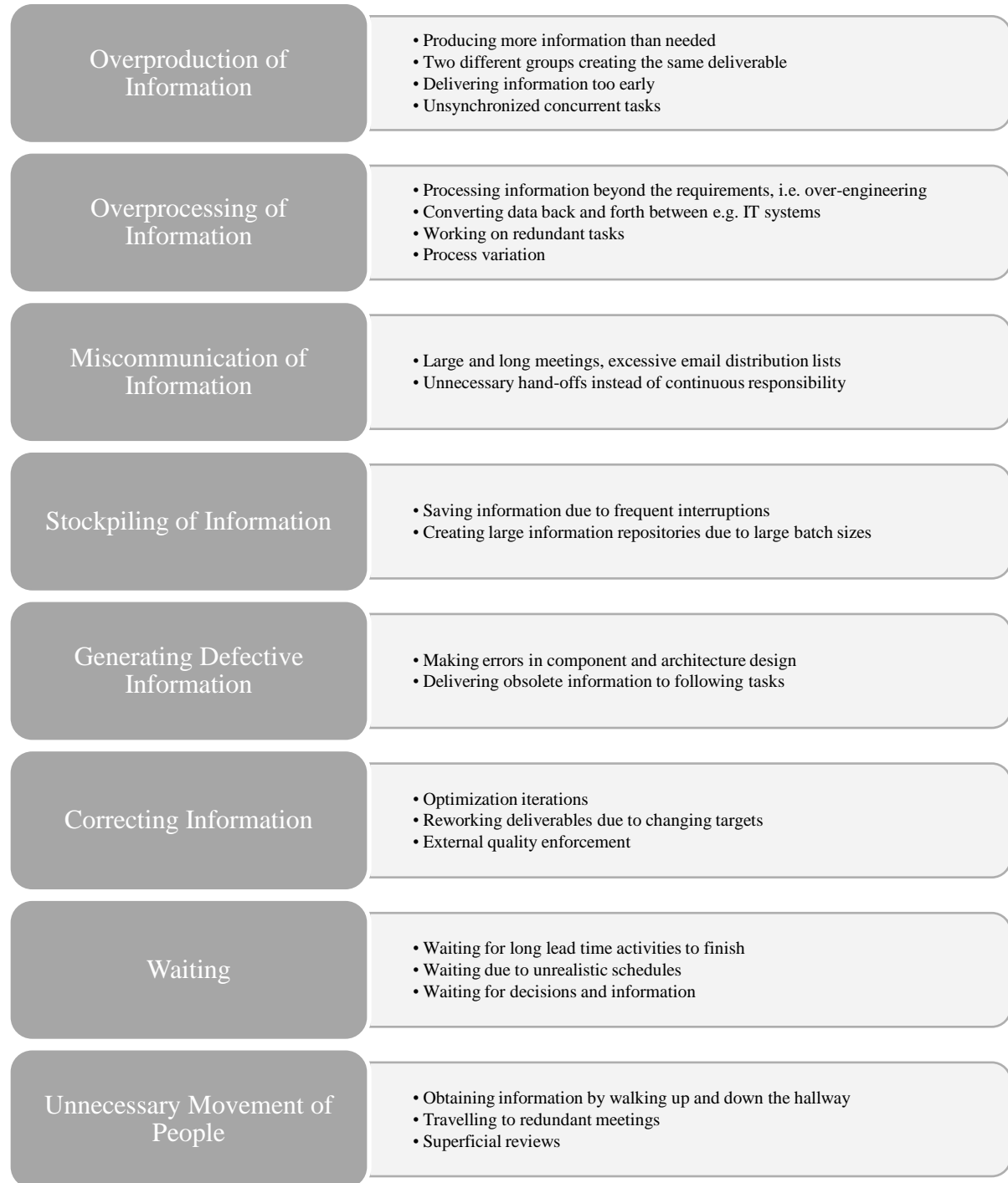
Figure 15: The Seven Manufacturing Wastes in the Perspective of Design and Engineering, derived from (Ćatić & Vielhaber, 2011; McManus, 2005; Morgan & Liker, 2006; Oehmen & Rebentisch, 2010)
