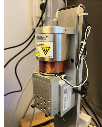
Fig. 7. Experimental setup of the voice-coil drive with 1 DOF.
