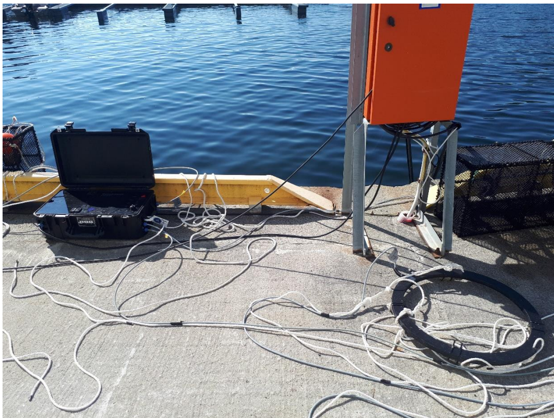
Figure 8: PIT-tag antenna (circular shape on the right) and tag-reader (box to the left) that were used at the pier to detect PIT-tagged goldsinny and corkwings.
