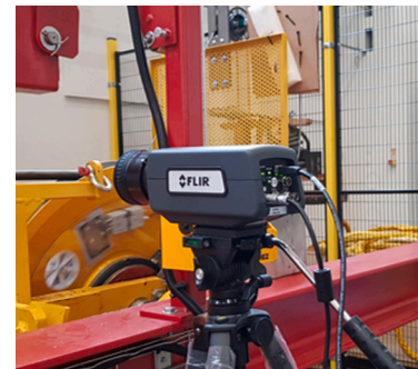
Fig. 5. FLIR A6753sc thermal camera at CBOS machine test sheave.
