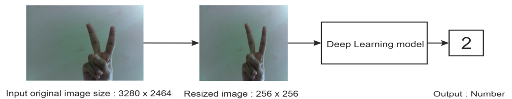
Figure 2. The classification (digit recognition) task used in the proposed end to end system for contactless authentication. The architecture details of the deep learning model are shown in Figure 4 and in Table 5.
