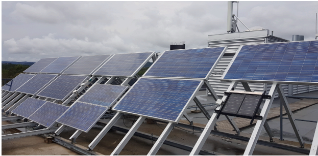
Fig. 1. Experimental setup 1 containing the poly c-Si PV modules used in this study. The full experimental details are described in (Paudyal and Imenes, 2019).
