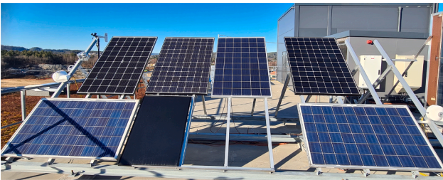
Fig. 2. Experimental setup 2 with PV modules from various technologies evaluated in this study.
